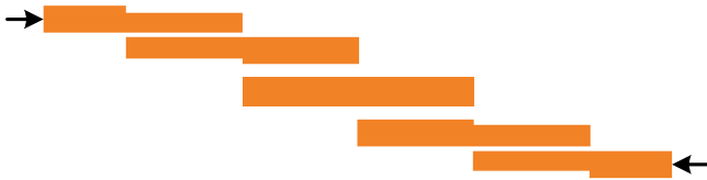
Fig. 5. The structure of the microstrip bandpass filter under study.
