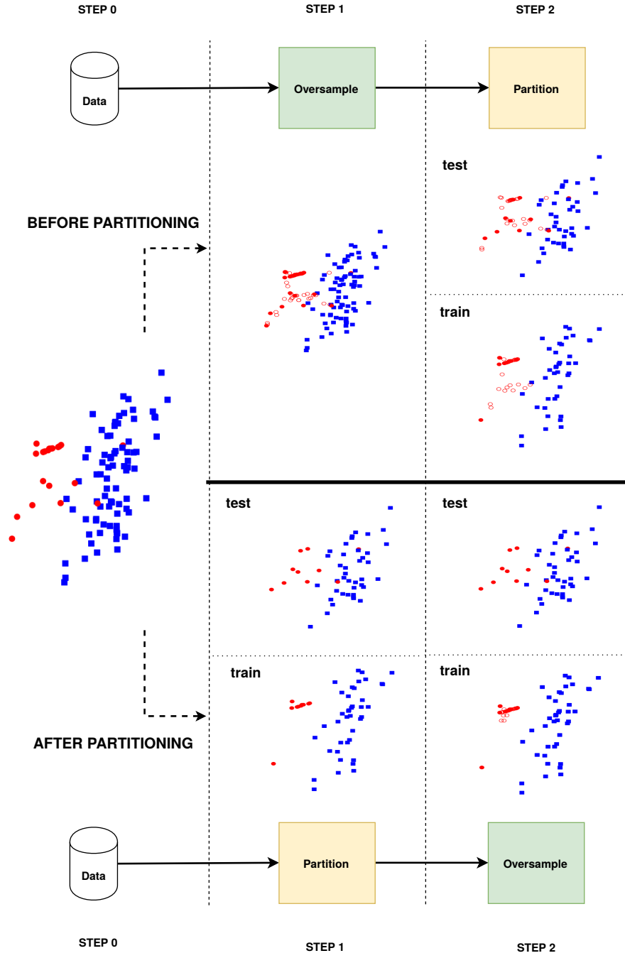
Fig.1. Comparing the impact of applying over-sampling prior to data partitioning to applying over-sampling after data partitioning on a two-dimensional classification problem.
