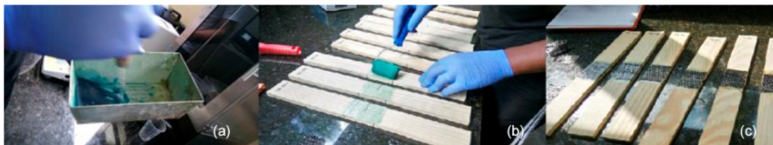
Figure 4: Roller for uniform spreading of bicomponent epoxy adhesive on the surfaces of fissured test specimens (a), dispersion of the resin in the regions of fixation of the composite (b), composite fixed to the wood specimens of Pinus elliotti . (c).
