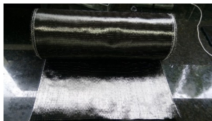
Figure 3: Unidirectional carbon fiber Viapol Carbon CFW 300.
