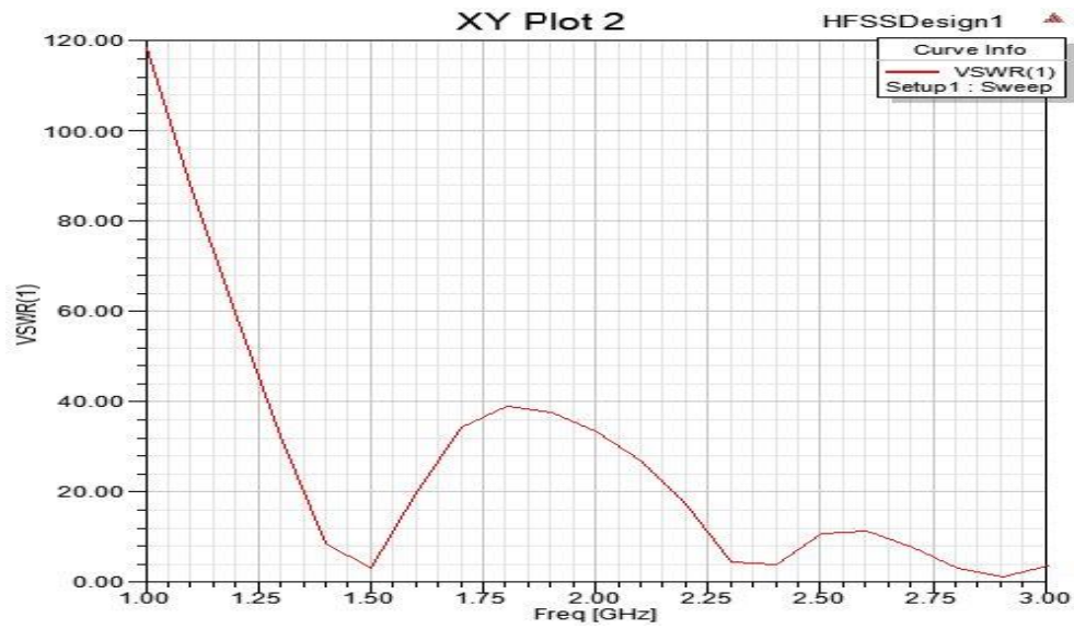
Figure 3: VSWR plot for 1.5GHz.
