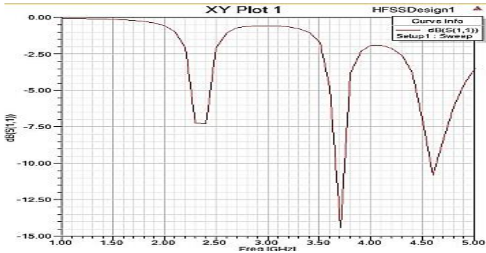
Figure 6: S-Parameter plot for 2.4 GHz.
