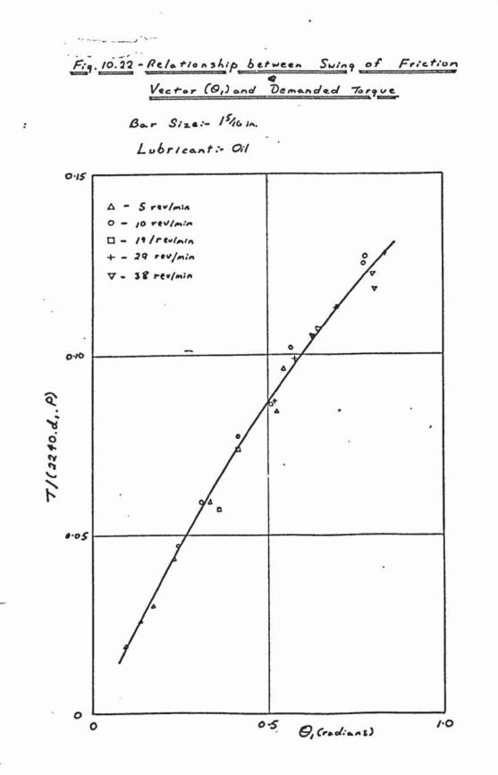
Fig. 10.23 - Dependence of Reduction in Drawing Force on Swing of Friction Vector (01)
