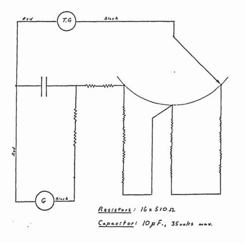
Fig. 6.1 - Circuit Diagram for Measurement of Rotational Speed
