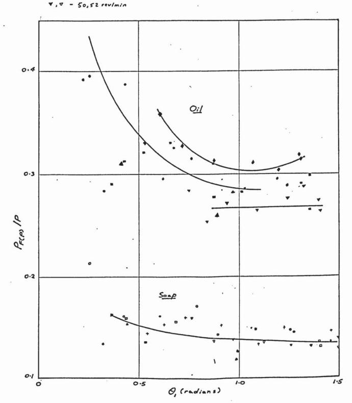
Fig.10.50- Component of Drawing Force due to Friction. Calculated from Reduction in Drawing Force, assuming n=1.
