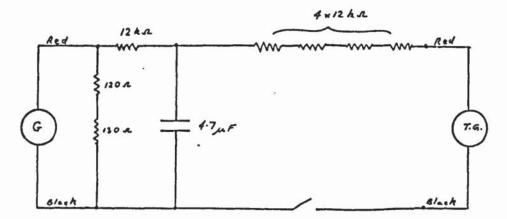
· Fig. 6.2 - Circuit Diagram for Measurement of Drawing Speed
