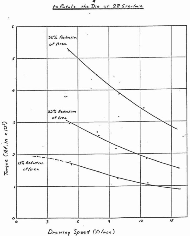
Fig. 9.4- Effect of Drawing Speed on Torque Required to Rotate the Die at 28.5 rev/min.
