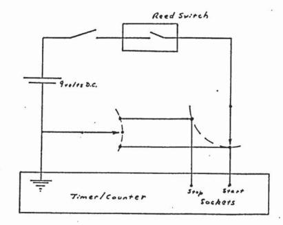
Fig. 7.1(a) - Circuit for Calibration of Rotational Speed Transducer
