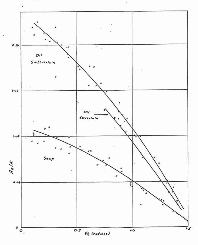
Fig. 10.40 - Influence of Speed and Friction Parameters on Rotational Speed of the Undrawn Bar
