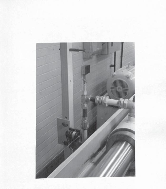
Plate 3 :- ARRANGEMENT OF DRIVE TO DRAWING-SPEED TACHOGENERATOR
