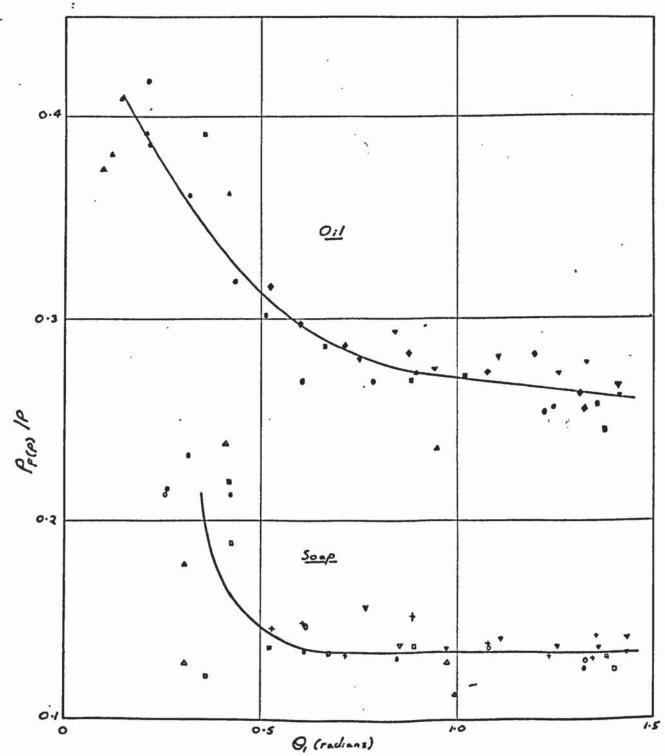
Fig. 10.49 - Component of Drawing Force due to Friction.
