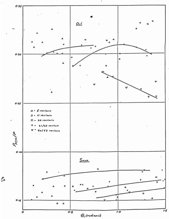
Fig. 10.45 - Component of Drawing Force due to Fristion.
