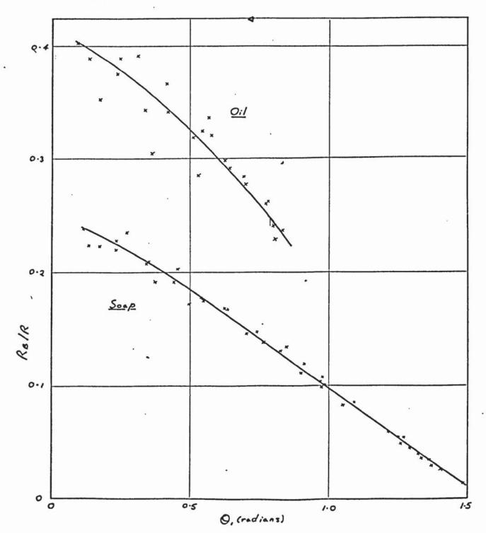
Fig. 10.42 - Component of Drowing Force due to Friction,
