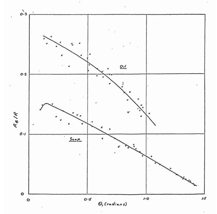
Fig. 10.41. Influence of Speed and Friction Parameters on Rotational Speed of the Undrawn Bar.
