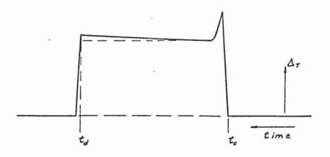
Fig. 10.13 - Form of Torque Record sometimes obtained When drawing with Soop
