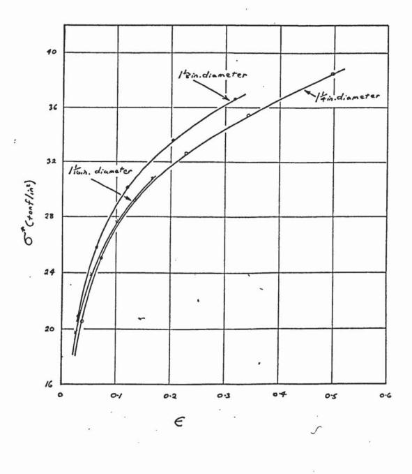
Fig. 9.1 - True Stress-Strain Curves for Material used in Series 1
