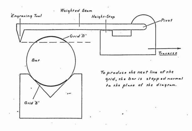
Fig. 10.3. - Mode of operation of 'Tracelet' Mechanism.
