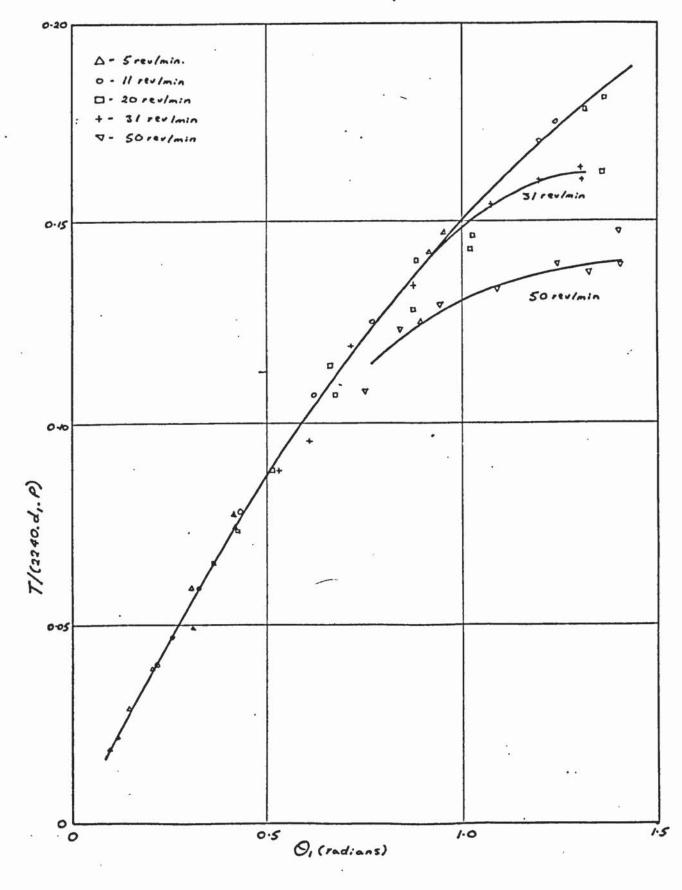
Fig. 10.19 - Relation ship between Swing of Friction Vector (0,) and Demanded Torque
