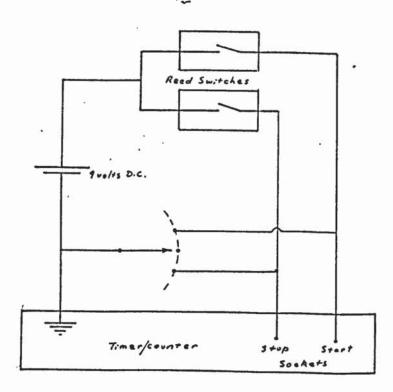
Fig. 7.1(6) · Circuit for Colibration of Drawing Speed Transducer
