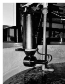
Fig. 6. Pallet dispenser distributor
