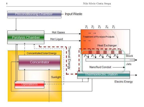
**Fig. 2:** The complete scheme of the proposed thermodynamic engine. Note the cicle of energy with a thermoelectric station feeding continually the usine as well as it is powered by solar energy (from Serpa's Ph.D. thesis in French [44]).
