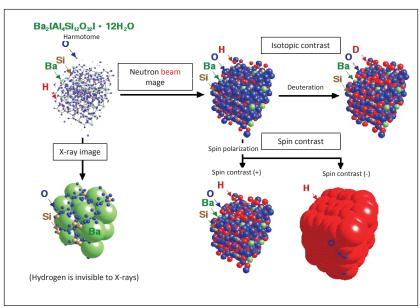
Figure 6: Schematic Representation of Structural Analysis Using Neutron Beam Source: reference<sup>[13]</sup>
