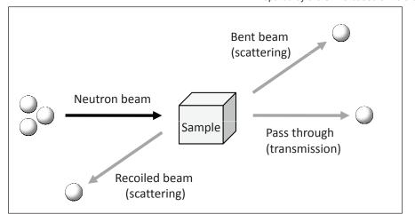
Figure 2: Material Analysis Using Neutron Scattering and Transmission Prepared by the STFC based on reference<sup>[4]</sup>
