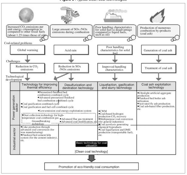
Figure 6 : Typical clean coal technologies
