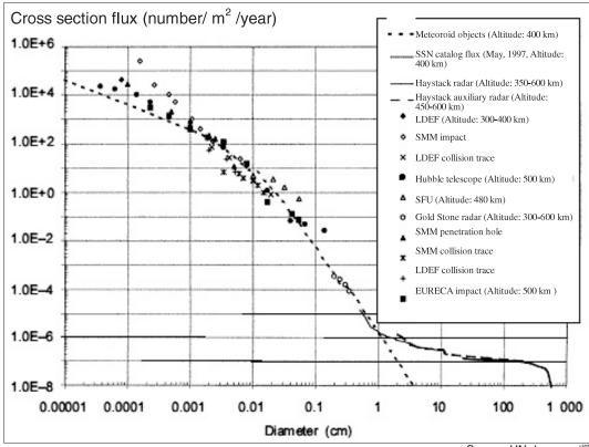
Figure 7 : Space Debris Flux Model
