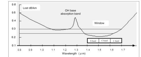
Figure 1 : Optical fiber transmission loss bands and optical fiber amplifier operation frequency
