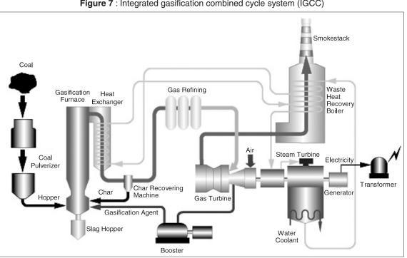
Figure 7 : Integrated gasification combined cycle system (IGCC)
