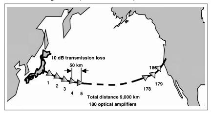
Figure 3 : Repeaters for the Transpacific Cable
