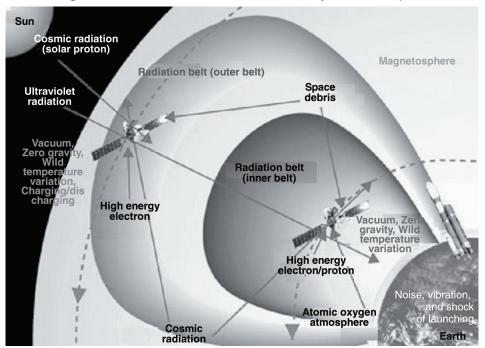
Figure 2 : Radiation Environment and Cosmic Ray Hazards in Space
