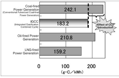
Figure 8 : CO<sub>2</sub> emissions per unit power generated
