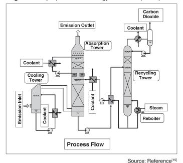
Figure 8 : CO<sub>2</sub> separation technology for thermal power plants
