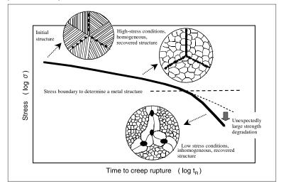
Figure 5 : Stress dependency and effects on creep strength by the microstructure of heat resistant steel during high-temperature creep<sup>[19]</sup>
