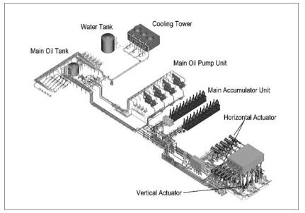
Figure 4 : Shaking table and actuator system
