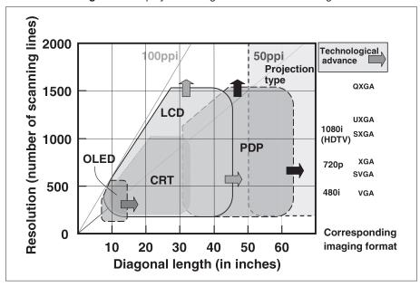
Figure 2 : Display technologies and their useful ranges
