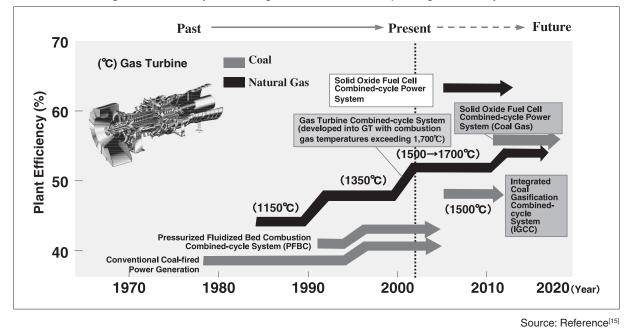
Figure 7 : Efficiency of natural gas-fired and coal-fired power generation systems
