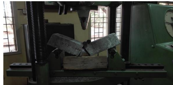
Figure: 4 Flexural Strength Test
