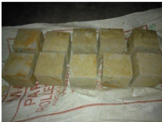
Figure: 6 Sulphate Attack Test
