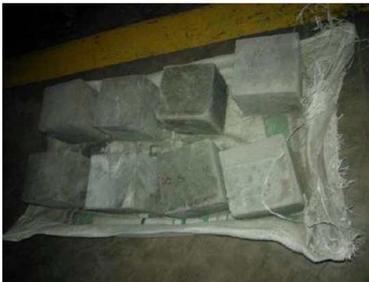
Figure: 8 Chloride Attack Test
