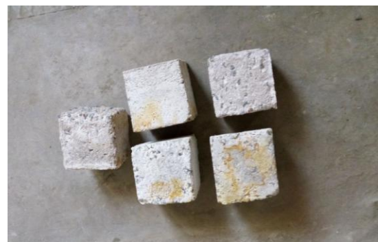
Figure: 10 Acid Attack Test
