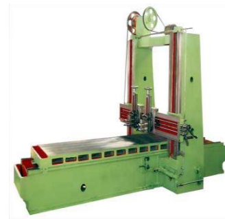
Figure: 1 Photographic view of a planning machine
