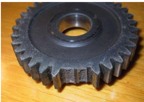
Figure: 2 Damaged gear
