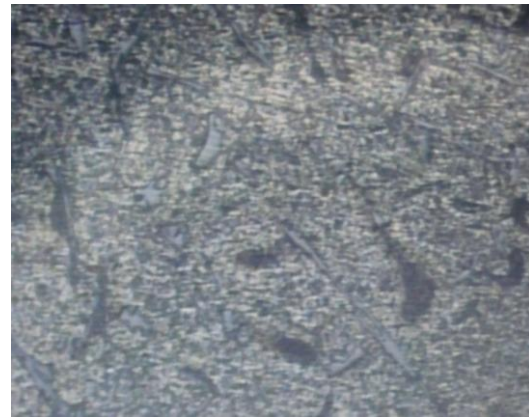
Figure: 8 Microstructure of 2.5% Al_2O_3
