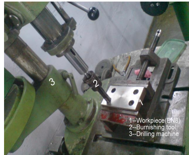
Figure: 1 Burnishing operation in drilled holes
