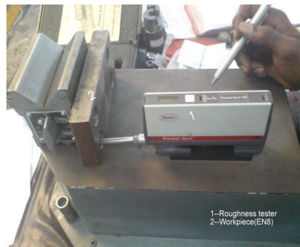
Figure: 2 Checking of roughness
