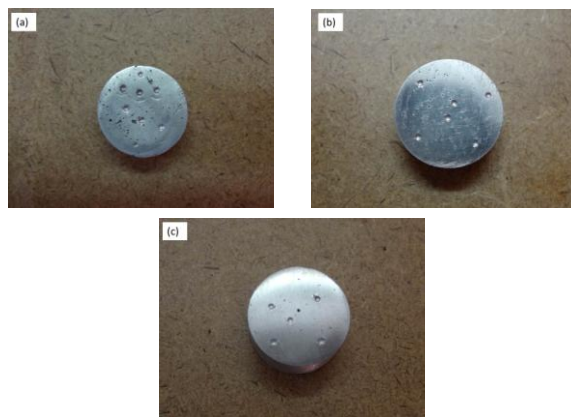
Figure: 2 Visual Investigation of Porosity corresponds to (a) MMNC with 1% Al 2 O 3 , (b) MMNC with 1.5% Al 2 O 3 , (c) MMNC with 2.5% Al 2 O 3 .
