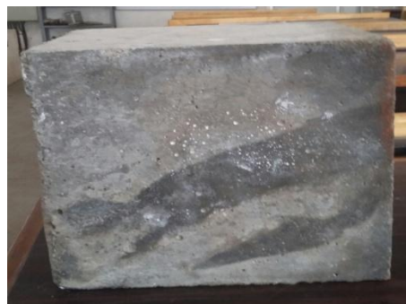
Figure: 9 Cube after sulphate attack
