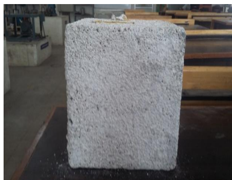
Figure: 8 Cube after acid attack
