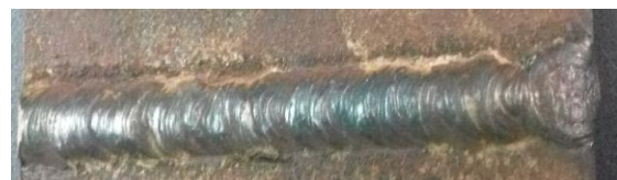
Figure: 5 Air welding bead appearance
