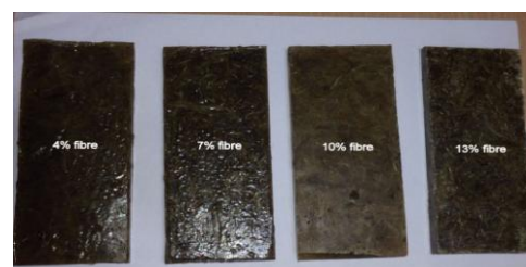
Figure: 1 Samples of the hemp fibers with different fiber percentages by weight
