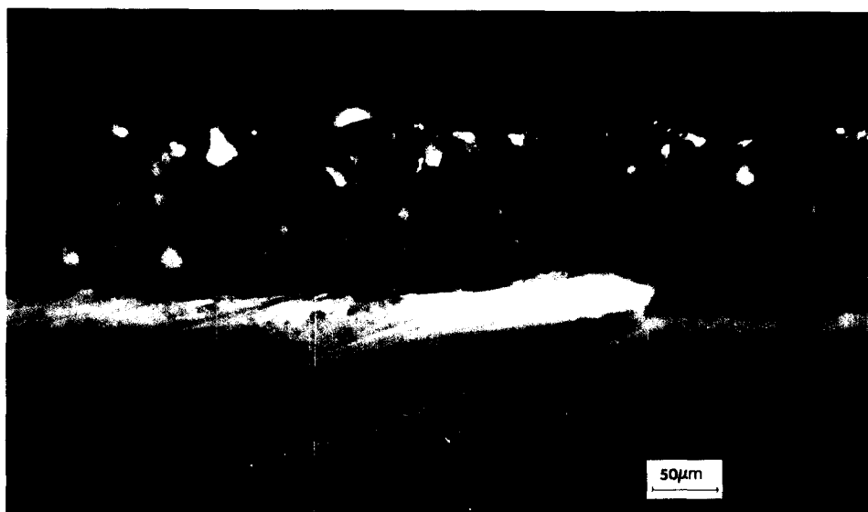
FIG. 9. Photomicrograph of the adhesive layer and one hand-sanded adherend showing lack of adhesive penetration of vessels and fibers.
