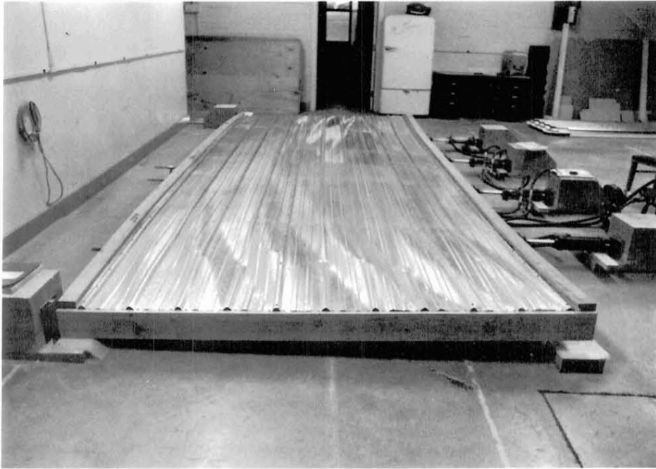
FIG. 2. Loading system and end supports. Also shown are 5 to 6 ripples starting from the ends and propagating towards the center.
