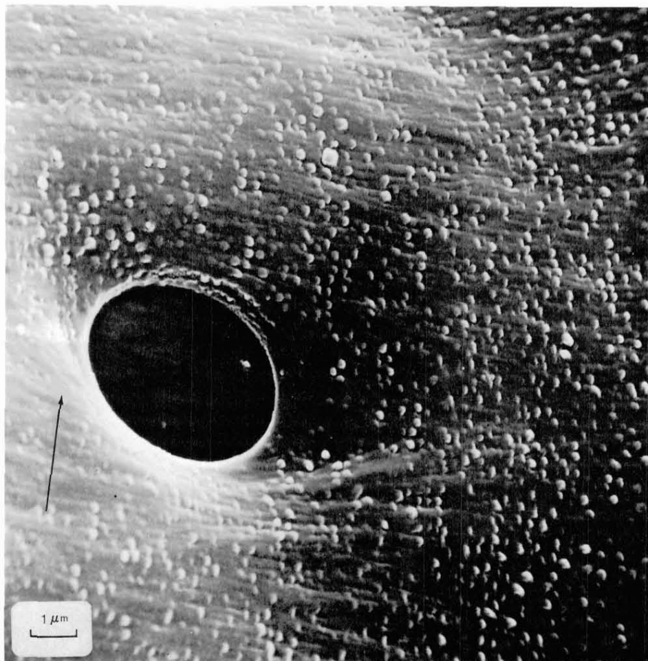
FIG. 1. An SEM micrograph of the warty layer of a water-extracted red pine heartwood tracheid (long arrow = fiber axis).
