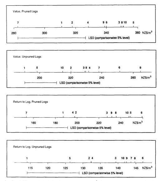
FIG. 3. Clonal differences in intrinsic value (average value per  $m^3$  of output) and return-to-log (value of output per  $m^3$  of input) for NZ Visual grades.
