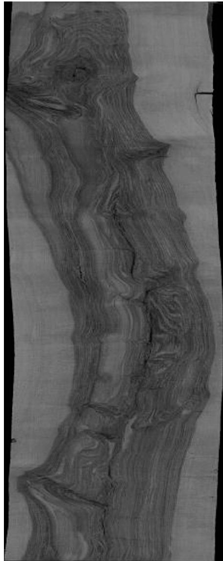
Figure 9. Example of a difference in color homogeneity between sapwood and discolored wood regions. Although sapwood is homogeneous in color, discolored wood presents different shades and creates a visual marble effect.
