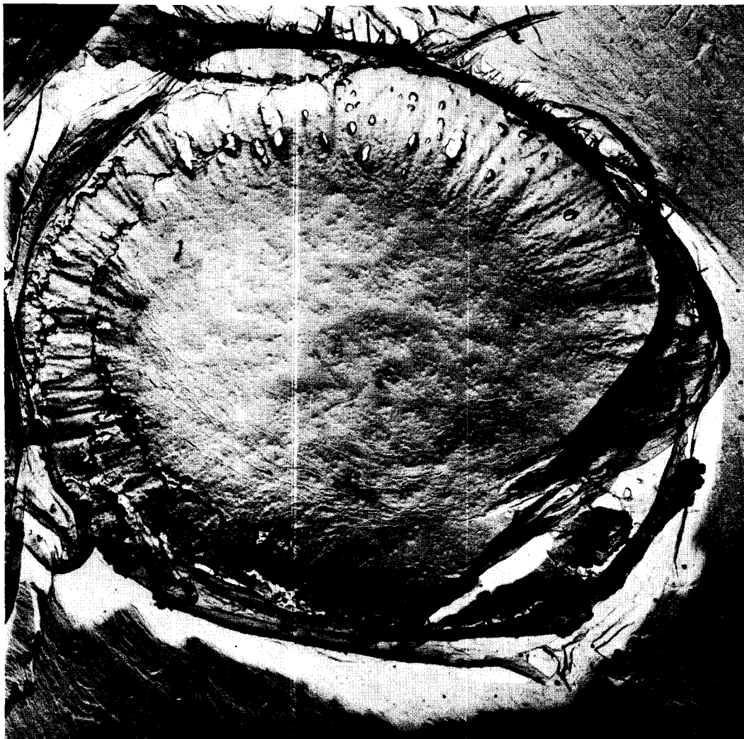
FIG. 5. Heavily encrusted bordered pit membrane observed in sinker heartwood of western hemlock. 7500 \times .
