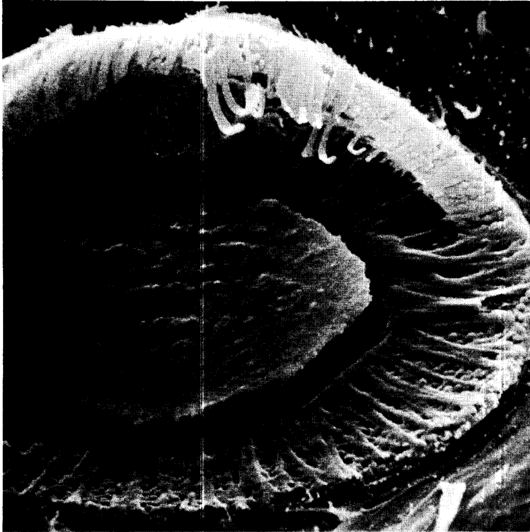
FIG. 12. Scanning electron micrograph of ruptured bordered pit membrane in acetone-extracted sinker heartwood. 13,000 \times .
