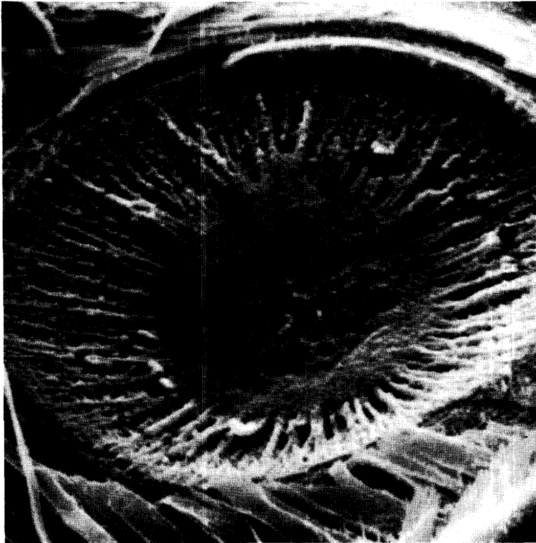
FIG. 4. Scanning electron micrograph of bordered pit membrane in normal heartwood of western hemlock.
