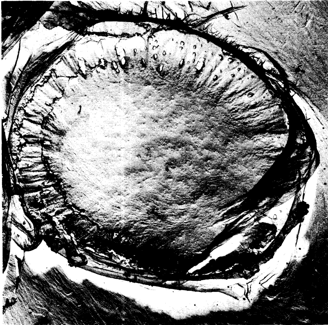
FIG. 6. Electron micrograph of bordered pit membrane in air dried wetwood of western hemlock. (This picture is supplied by Allen Doerksen, School of Forestry, Oregon State University.)
