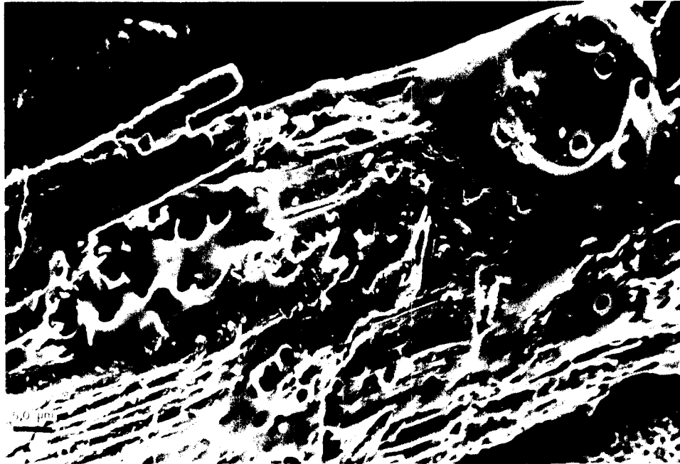
FIG. 9. Scanning electron micrograph of southern pine wood extracted at 100 C and 27.6 MPa.
