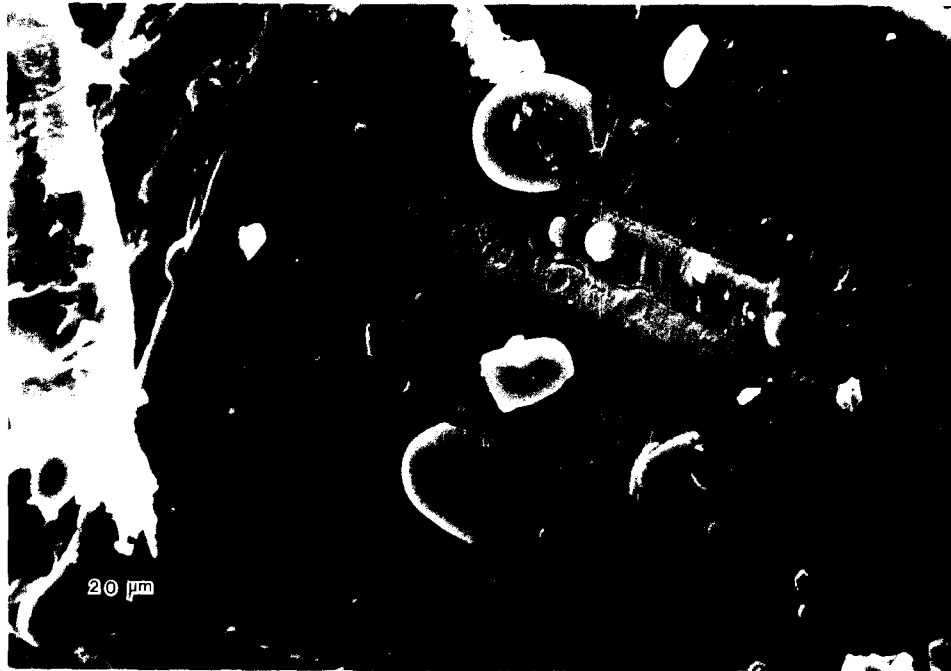
FIG. 8. Scanning electron micrograph of southern pine wood extracted at 40 C and 10.4 MPa.
