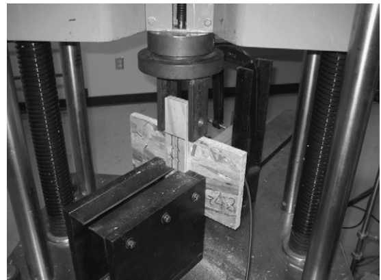
Figure 3. Test setup for evaluating lateral resistance load of face-to-face two-row multistaple joints in oriented strandboard materials.
