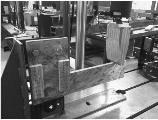
Figure 4. Test setup for evaluating bending moment resistance of L-shaped two-gusset-plate joints in oriented strandboard materials.
