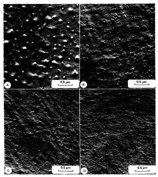
Fig. 4. Stages in treatment of balsam fir warty layer with DMSO at 150 C: A. 5 h, B. 10 h, C. 13.5 h, D. 15 h.
