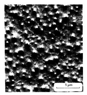
FIG. 3. Appearance of balsam fir warts after 35 h of exposure to 72% sulfuric acid at room temperature.
