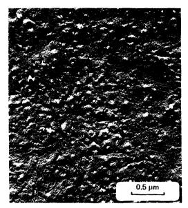
FIG. 5. Intermediate stage of balsam fir wart degradation by 30% hydrogen peroxide (at room temperature for 7 days). Note the "crater" morphology of residual wart material.
