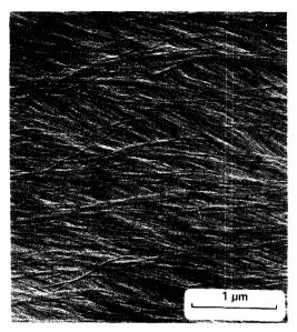
FIG. 7. Tracheid lumen surface of balsam fir after treatment with sodium chlorite followed by pectinase. Compare to Fig. 2 without pectinase treatment.
