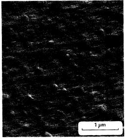
FIG. 2. Warty layer of balsam fir after treatment with 4.5% sodium chlorite, pH 4.0, at room temperature for 4 weeks.
