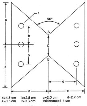
Fig. 2 Geometric dimensions of specimen.
