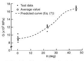
Fig. 3 Variation of shear modulus G with grain slope  $\theta$
