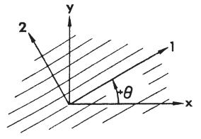
FIG. 1. Positive rotation of principal material axes (1 and 2) from geometric axes (*x* and *y*).
