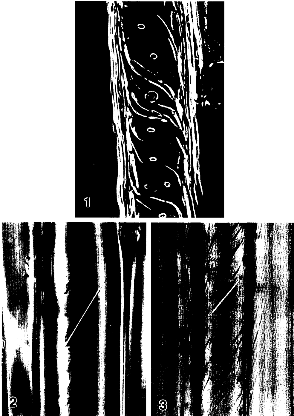
FIG. 1. Soft-rot cavities in a tracheid from a maceration prepared from a decayed block of southern pine. The cavities follow the microfibril angle in the S2 layer of the cell wall. Soft-rot cavities are also visible in a pit border forming a circular chain of cavities. 500 \times .
