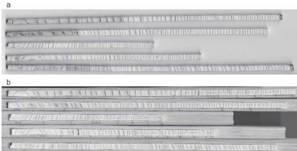
FIG. 4. Ponderosa pine cores (a) prior to peroxide bleaching pretreatment and (b) after bleaching. Direction of tree growth is from left to right.
