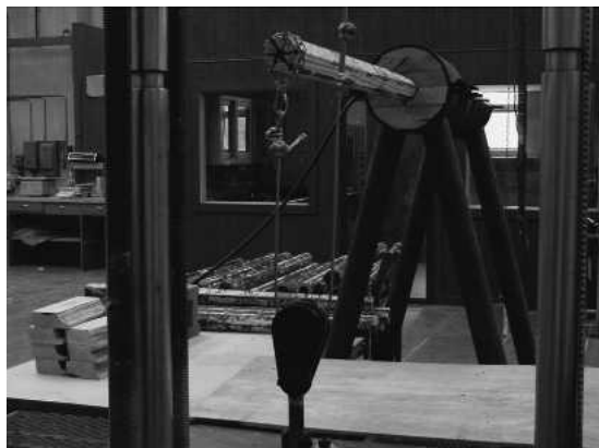
FIG. 5. A small-scale composite pole being tested in a RIEHLE machine.
