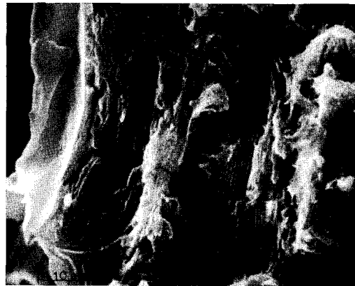
Fig. 21. The thick-walled cogwheel phellem of longleaf pine display multilayered cell walls traversed by pore or pit canals, and a lumen often containing extractive material (scanning electron micrograph, radial face).
