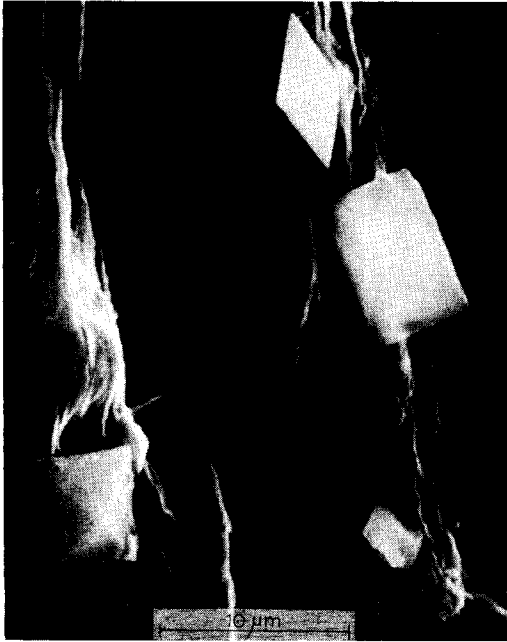
Fig. 15. Crystals of various shapes occur in the bark of trees (Red oak, Quercus rubra L., scanning electron micrograph, radial face).
