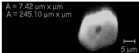
Figure 2. Cross-sectional areas of single bamboo fibers determined by confocal scanning laser microscopy.
