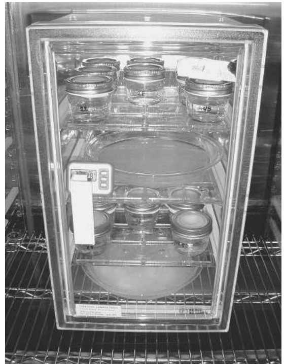
Figure 2. Cabinet with assembled diffusion cups during diffusion tests.
