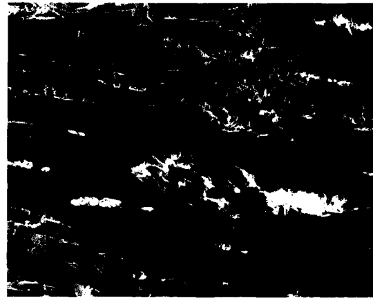
FIG. 6. Scanning electron micrograph of Douglas-fir veneer ( \times 200 ) in which wood fibers have been pulled away by the shearing action of the veneer-peeling process.
