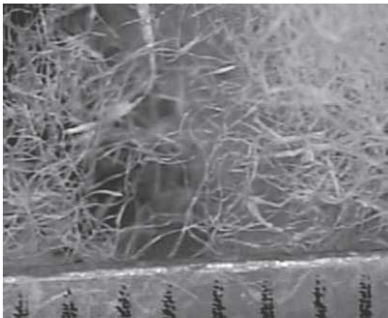
FIG. 3. A typical high porosity fiber mat with fibers that are loosely entangled to each other. Length scale indicates mm.
