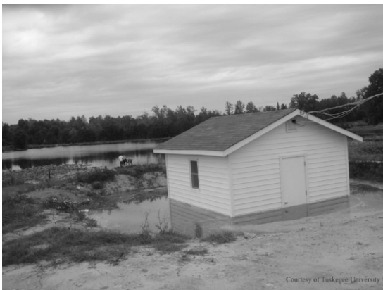
Figure 1. Flood unit built at Tuskegee University at flood stage. Unit is surrounded by 0.91 m of water from a nearby pond (in back of photograph). After 3 wk of flooding, the water was drained and the unit remained closed for an additional 3 wk prior to sampling.
