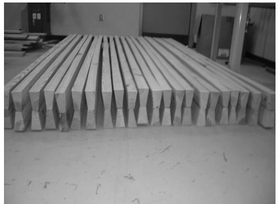
Figure 2. The completed 22 bowtie beams.
