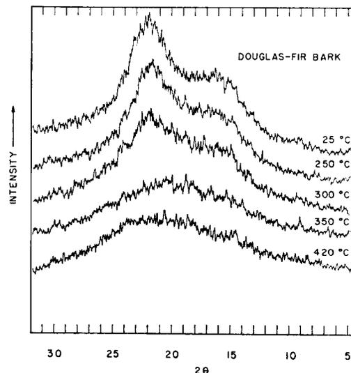
FIG. 7. X-ray diffraction pattern of Douglas-fir bark (powder).
