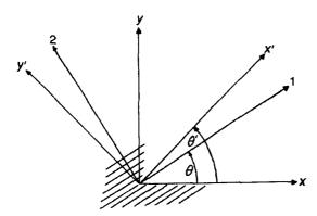
Fig. 1. Coordinate axes in principal material plane.
