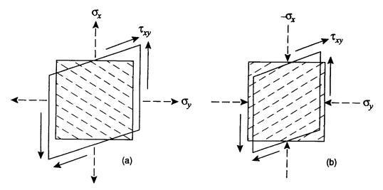
Fig. 8. Response of material elements with grain slope under pure shear loading: (a)  $+ \theta$ , (b)  $-\theta$ .
