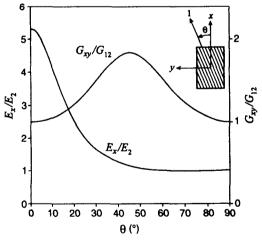
Fig. 5. Elasticity and shear moduli of Sitka spruce versus grain slope ( $E_1 = 11.800$  MPa,  $E_2 = 2.216$  MPa,  $G_{12} = 910$  MPa,  $v_{12} = 0.37$ ).
