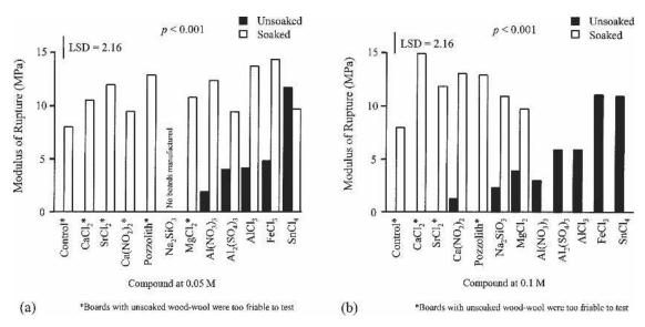
FIG. 1. Average MOR of wood-wool cement boards manufactured from unsoaked and soaked *A. mangium* wood-wool with accelerators applied at (a) 0.05 M and (b) 0.1 M concentration.
