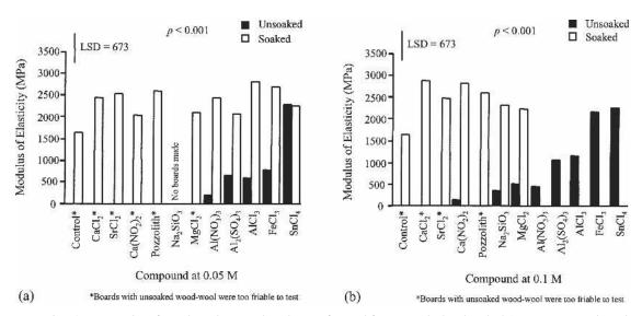
FIG. 2. Average MOE of wood-wool cement boards manufactured from unsoaked and soaked *A. mangium* wood-wool with accelerators applied at (a) 0.05 M and (b) 0.1 M concentration.
