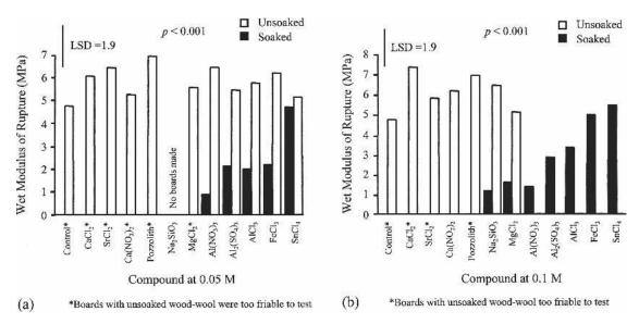
FIG. 3. Average wet MOR of wood-wool cement boards manufactured from unsoaked and soaked *A. mangium* wood-wool with accelerators applied at (a) 0.05 M and (b) 0.1 M concentration.
