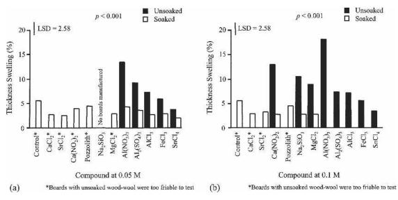
FIG. 4. Average thickness swell of wood-wool cement boards manufactured from unsoaked and soaked *A. mangium* wood-wool with accelerators applied at (a) 0.05 M and (b) 0.1 M concentration.
