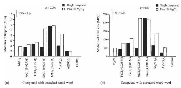
FIG. 5. The effect on (a) MOR and (b) MOE of combining selected accelerators with 0.05 M (1%)  $MgCl_2$  compared to adding the accelerators on their own to wood-wool cement boards made from unsoaked wood-wool.
