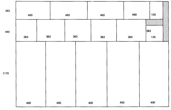
FIG. 5. Cutting pattern 2 (98.5% recovery).
