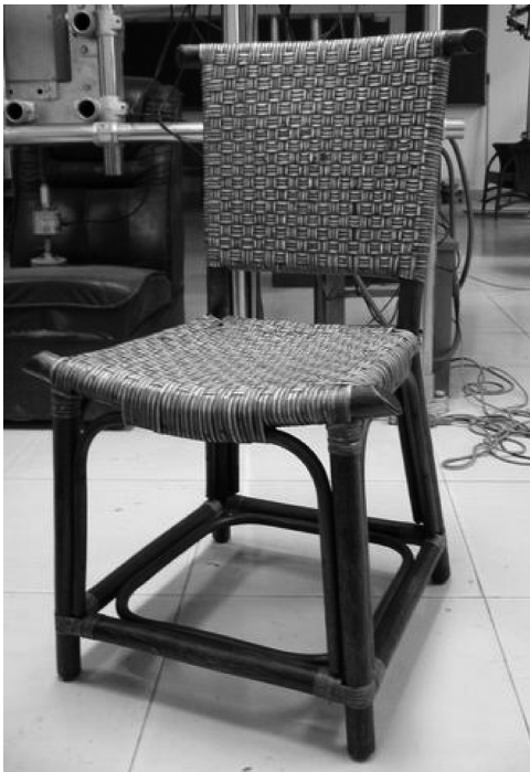
Figure 4. A rattan chair used for evaluation of load-deflection behavior of its seat foundation surface subjected to cyclic vertical loads.
