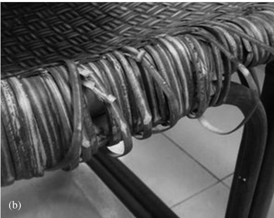
Figure 9. Two typical failure modes in seat foundation surfaces of rattan chairs subjected to vertical cyclic loads: (a) nonrecoverable concaved deformation and (b) loosen and broken strips along frame edges.
