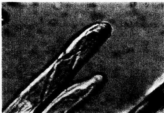
FIG. 9. Soft-rot cavities growing in a helical orientation in the tip of a southern pine tracheid. From Anagnost et al. (1999).
