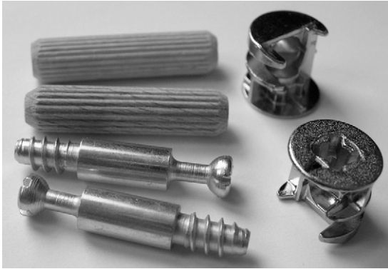
Figure 1. Cam fasteners (metal connecting bolts, cam housings) and multigrooved wooden dowels used in tests.
