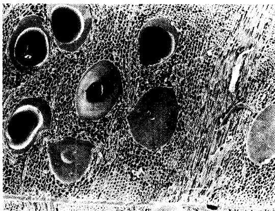
FIG. 6. Red oak, very slight damage near to the vessels filled by adhesive is noted, 2-mm jointed knife-planed specimen (SEM micrograph).
