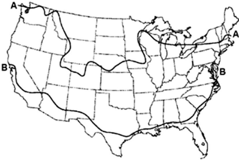
Figure 6. (a) The northern limit of recorded damage done by subterranean termites in the United States; (b) the northern limit of damage done by dry-wood termites (Moore 1979). Note: Termite damage has also been noted in southern British Columbia and Ontario, Canada (PI Morris, FPInnovations, Vancouver, British Columbia, Canada).
