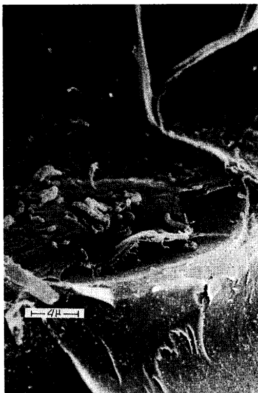
FIG. 7. Bordered pit structure of the split radial surface of redwood sapwood. Solvent-exchange technique used achieved poor results. Note bacteria on the pit torus. (2100 \times )
