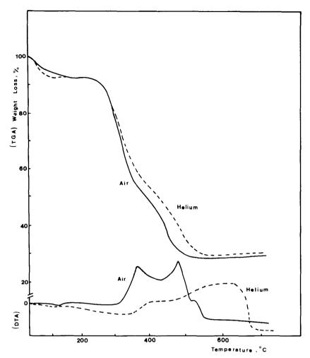
Fig. 4. DTA and TGA thermograms for rice hulls under oxidized and inert atmosphere.
