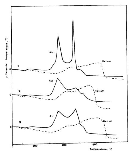
Fig. 1. DTA thermograms for nonwoody materials under oxidized and inert atmosphere.
