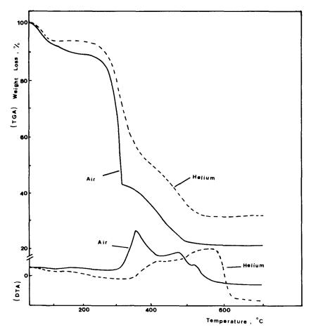
Fig. 3. DTA and TGA thermograms for rice straw under oxidized and inert atmosphere.
